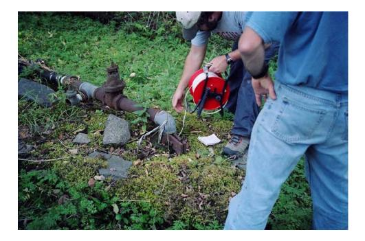
**Photograph 4:** Village Well 4. Performing a manual water level measurement with an electronic water level meter through a port at top of well cover.
