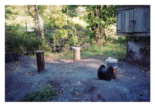
**Photograph 5:** Fleischmanns Village Well 1A with transducer/data logger installed (cable spool adjacent to well). Well in background is Village Well 1 (out of service). Emory Brook is just behind the brush, approximately 10 feet behind Well 1, and flows right to left in the picture.
