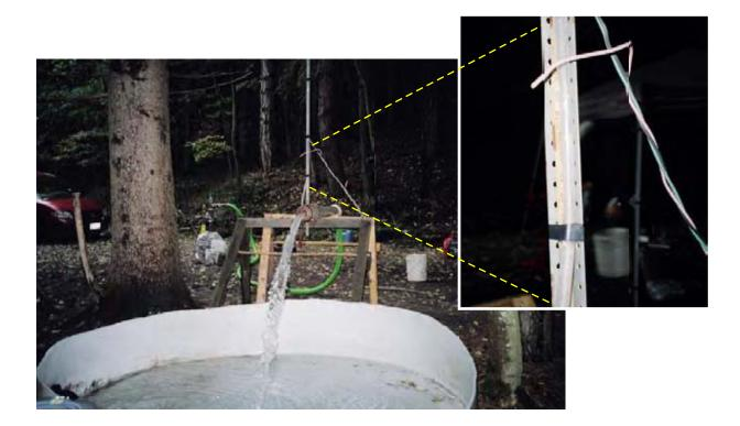
**Photograph 1:** Water discharging from well K4 through circular weir plate into large receptacle to prevent discharge to the land surface near the wells, to reduce the potential for erosion, to facilitate manual checking of discharge rates, and allow for sample collection. The water drains from the receptacle via two four-inch diameter plastic pipes. **Inset:** close up view of manometer tube used as a check on discharge rates.
