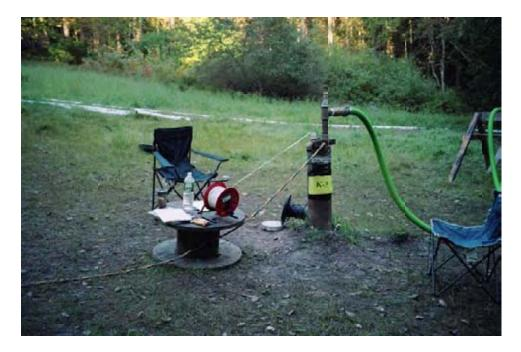
**Photograph 3:** K3 Well head. Ball valve for controlling discharge rate is located just prior to green discharge hose. Two stilling tubes, one for manual water level readings and one for a downhole data logger/pressure transducer, were installed in the wells. Hose bib at top is for attaching the MPA sampling kit.
