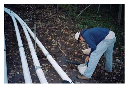
**Photograph 9:** Measuring water quality of K1 Spring. Spring yield was measured with a calibrated bucket and stopwatch. The K1 Spring vent is at the base of the steel well point (between plastic pipes). The flow from the spring was dammed and conducted through the dam by a plastic pipe.
